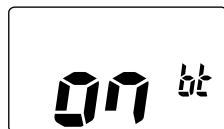
Battery voltage indication ON
